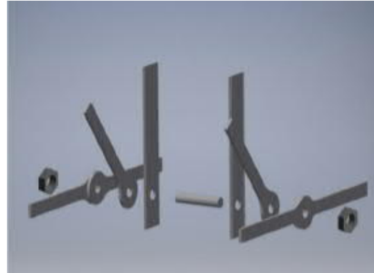
Image 9: Model of a Disassembled Pin Connection
